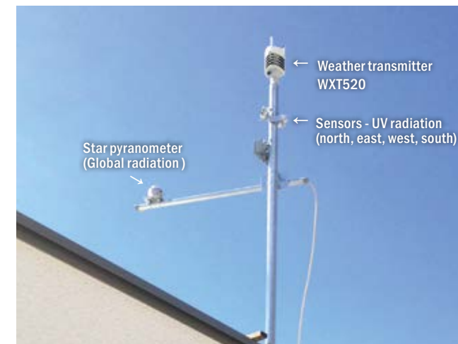
Weather transmitter and radiation meter on the roof of measurement house no. 8
