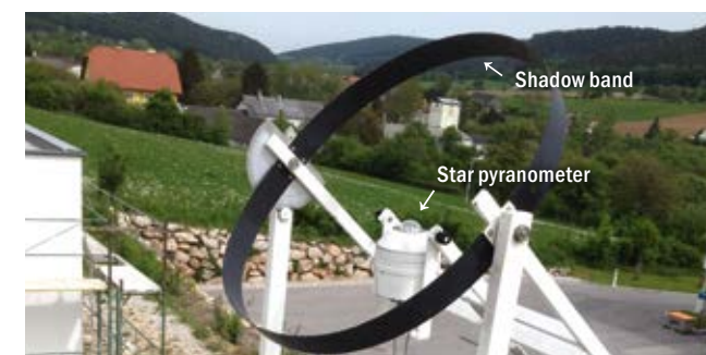
Star pyranometer with shadow band for measuring the diffuse radiation component of global radiation
