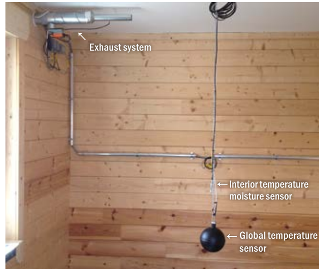
Moisture and global temperature sensor (shown here in the timber block house)
